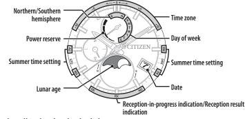
• A solar cell is placed under the dial.
